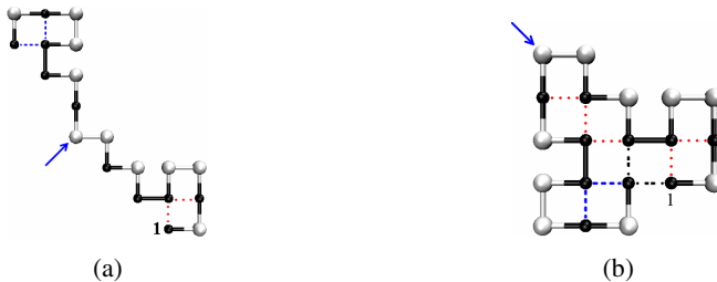
Fig. 4. An example of the mutation operation [46]. Dotted lines indicate TN. Residue number 11 is chosen randomly as the pivot. For the move to apply, a 180^\circ rotation (among a number of possible degree of freedom defined by the model configuration) alters (a) with F = -4 to (b) F = -9 . '→' indicates the mutation residue.
